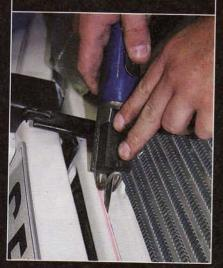
Space intercooler back 20mm using suitable spacer and tighten bolt.
