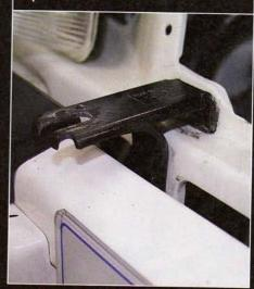
13 If necessary trim front panel to allow room for fans.
