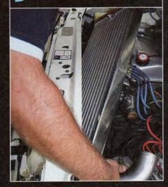
**10** Secure both cooling fans to intercooler using clips provided.
