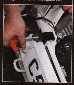
Using 20mm spacers, bolt radiator back into place.
